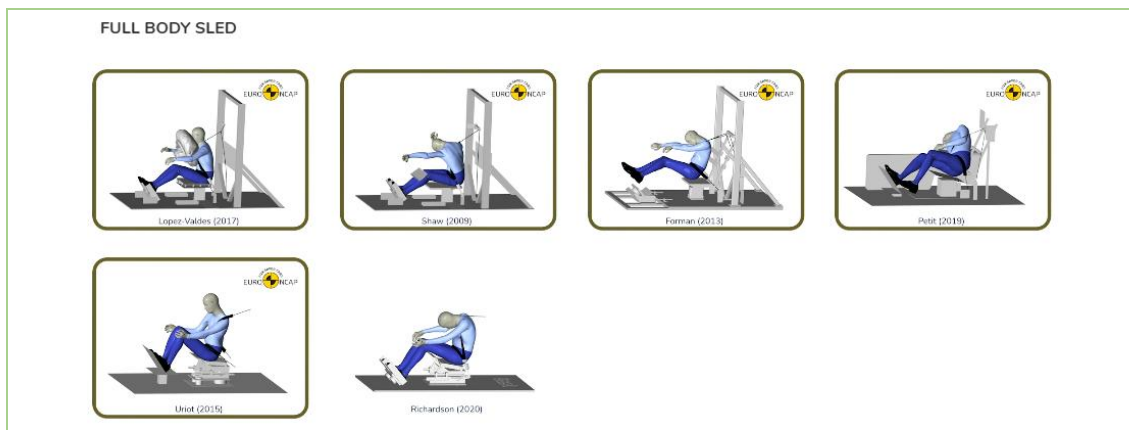
Configuraciones de ensayo modelo completo de HBM Connect 50th Male (Fuente: www.humaneticsgroup.com/products/virtual-models/hbm-connect )
