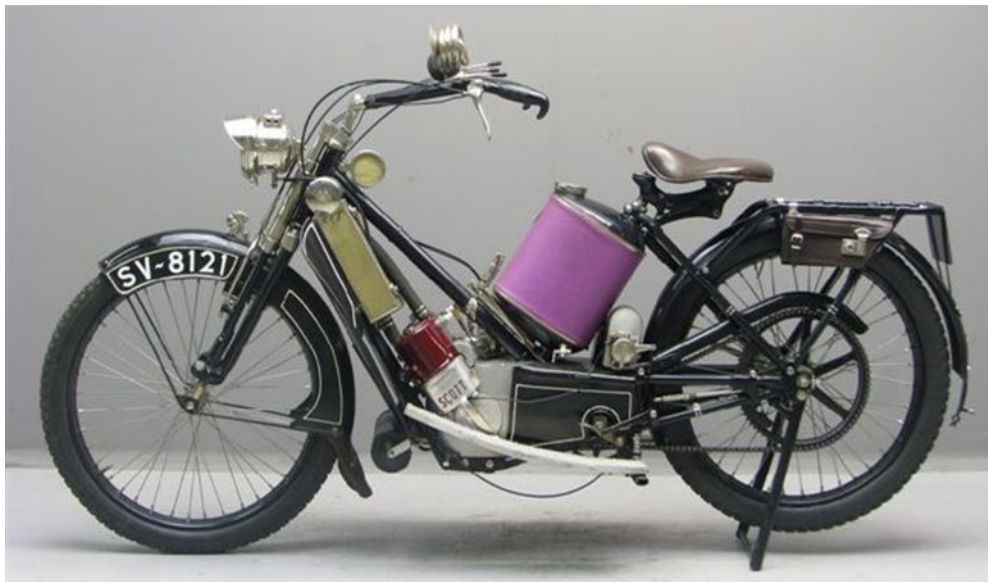
1924.- Scott Super Squirrel (R. U.) 498 cm 3 - 22 CV a 5500 rpm
