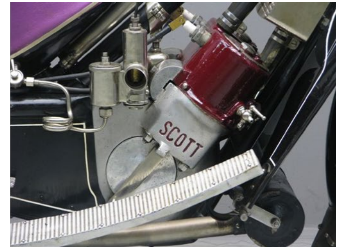
1924.- Scott Super Squirrel (R. U.) 498 cm 3 - 22 CV a 5500 rpm
