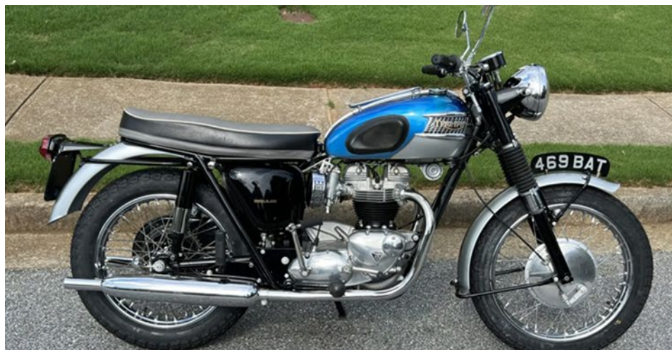
1960 Triumph Bonneville T120R 650 cm 3 – 47 CV a 6500 rpm
